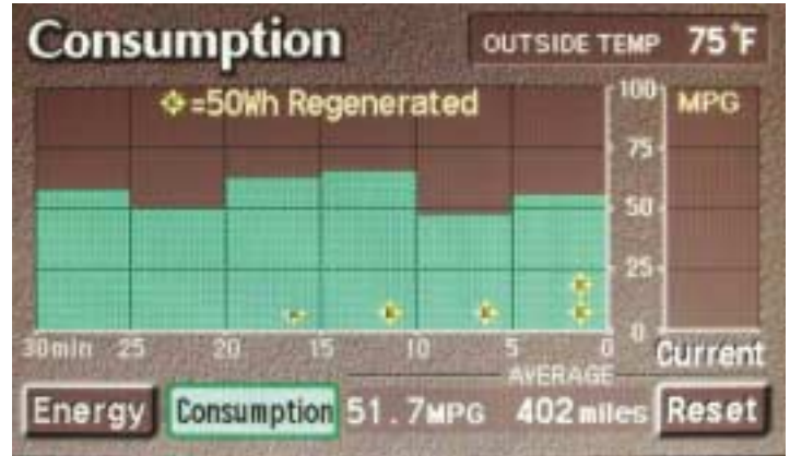
This fuel gauge from a Toyota Prius hybrid vehicle shows the energy consumption, power regeneration, and fuel economy for this trip (51.7 mpg).
